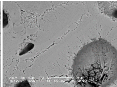
Figure 10. BSE image (1 h at 900°C, 10 sec etching).
