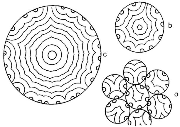
Figure 6 Change of mode and dimensionality of growth of athermal crystalline nuclei in glass grains with different grain radius  $R_0$ : (a) Small (dust-like) grains: three-dimensional growth,  $n=3$ , (b) medium sized glass grains:  $3 > n > 1$  and (c) large sized grains:  $n \approx 1$  (schematically).
