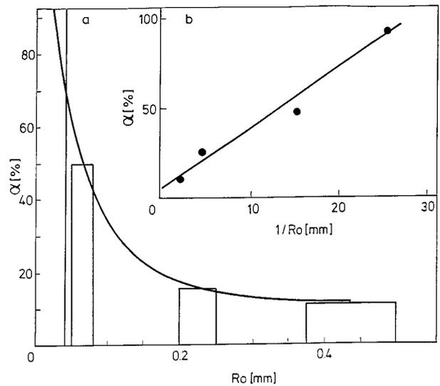
Figure 10 Overall crystallization of different fractions of  $\text{NaPO}_3$  glass semolina samples at constant time of heat treatment (1.5 h) at  $302^\circ\text{C}$ . (a)  $\alpha$  data as a function of grain radius  $R_0$ ; (b) the same data in coordinates  $\alpha$  vs.  $1/R_0$ .
