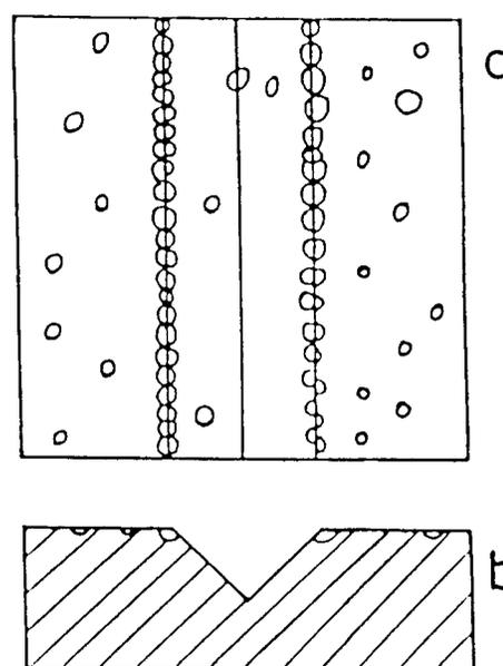
Figure 4 Preferred sites for the formation of crystalline clusters of the new phase accounting for the influence of elastic strains generated. Crystallization occurs along the edges of scratches and not in the grooves as should be expected in the case of heterogeneous nucleation. (a) Overview of the glass sample; (b) cross section of the same sample.
