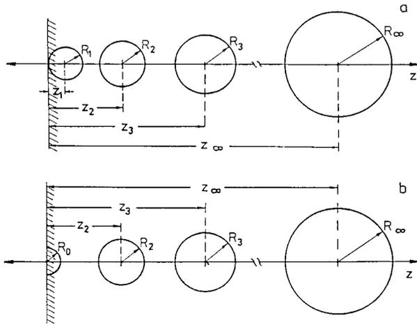
Figure 1 Change of shape and size of critical clusters in dependence on the distance from the free glass surface,  $z$ , for two hypothetical models with typical  $\Xi$  values: (a)  $\Xi = 1$  and (b)  $\Xi = 0$ . The lowest value of the work of formation of a critical cluster corresponds to a spherical cluster located tangentially to the interface for  $\Xi = 1$  (a) and to a hemisphere for  $\Xi = 0$  (b).
