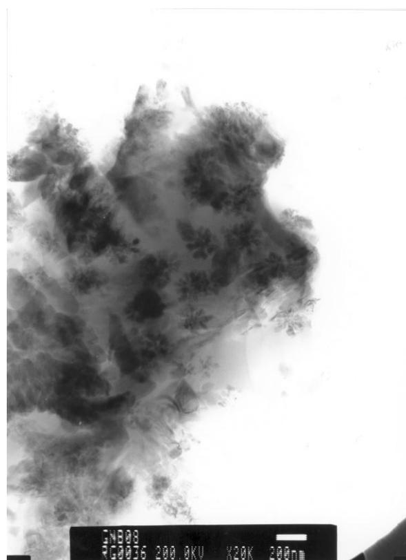
Fig. 5. TEM picture of J50 glass-ceramic at 142,000 magnification.
